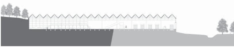
longitudinal section revealing long span structural requirements
