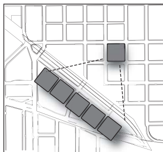
Sectionalizing masterplan to 200'x200' block, similar to urban scale of Portland
