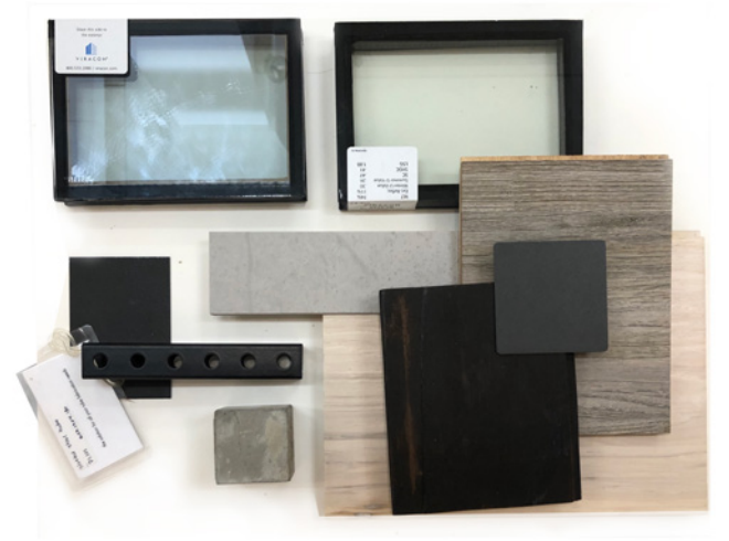
10 The materials chosen for the intervention include double-glazed glass, soft woods, ceramic tiles and site cast concrete; a reinterpretation of the original material palette.
