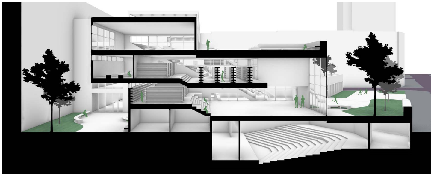
Top: A rendering of the double-height reading room, with its folding glass doors opening to extend the program out into the exterior patio space. Bottom: A section perspective cutting through the double-height reading room, demonstrating how the different program spaces extend out onto their exterior patios.
