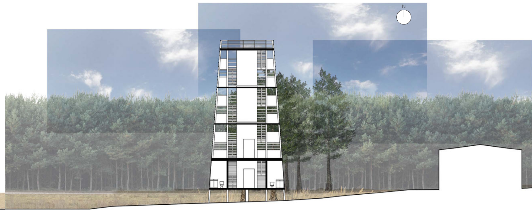
Top: A rendered plan of the pavilion's ground floor, labeling programmatic elements within the main pavilion and the tower. Bottom: Section cutting through only the tower portion of the pavilion. The change in wall angle from this direction highlights the complexity of the tower's form.
