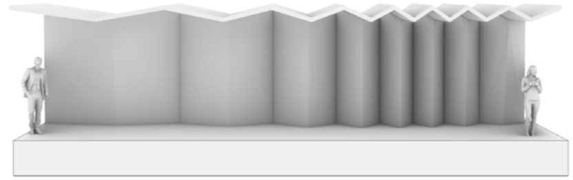
ZIP wall assembly - 'creased' to optimize structural performance
