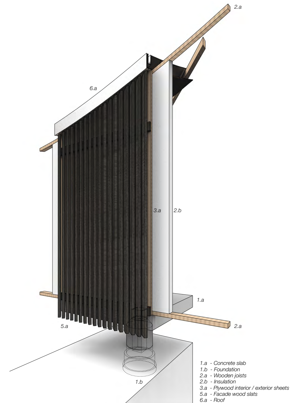
Structural Isometric and SIP chunk model.
