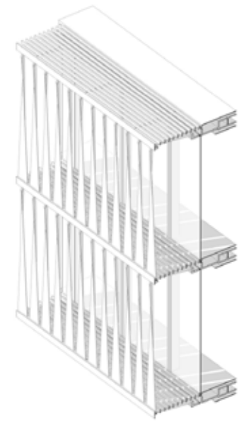
3d section of adaptive facade modeled in Rhino and Grasshopper in independent study with professor Jin Young Song
