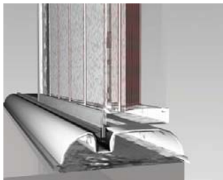
Head & Sill Section Detail Rhino & Flamingo
