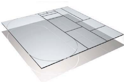
Zero waste: A coffee table fabricated from a 5'x 5' sheet of Baltic birch plywood. Wood-glued, stopped dado and rabbet joinery eliminate the need for hardware beyond two drawer hinges and a magnetic catch. Natural tung oil finish enhances the figured grain pattern and allows for simple cleaning and refinishing.
