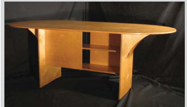
Zero waste: A coffee table fabricated from a 5'x 5' sheet of Baltic birch plywood. Wood-glued, stopped dado and rabbet joinery eliminate the need for hardware beyond two drawer hinges and a magnetic catch. Natural tung oil finish enhances the figured grain pattern and allows for simple cleaning and refinishing.
