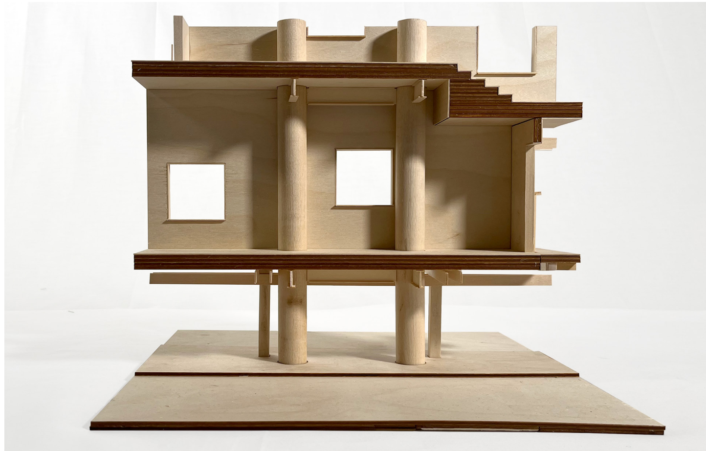
Above: A sectional model showing the way that the steel structure penetrates the CLT housing units. In a disaster event, the CLT is expected to be sacrificial, leaving the steel structure to support the refuge platform.
