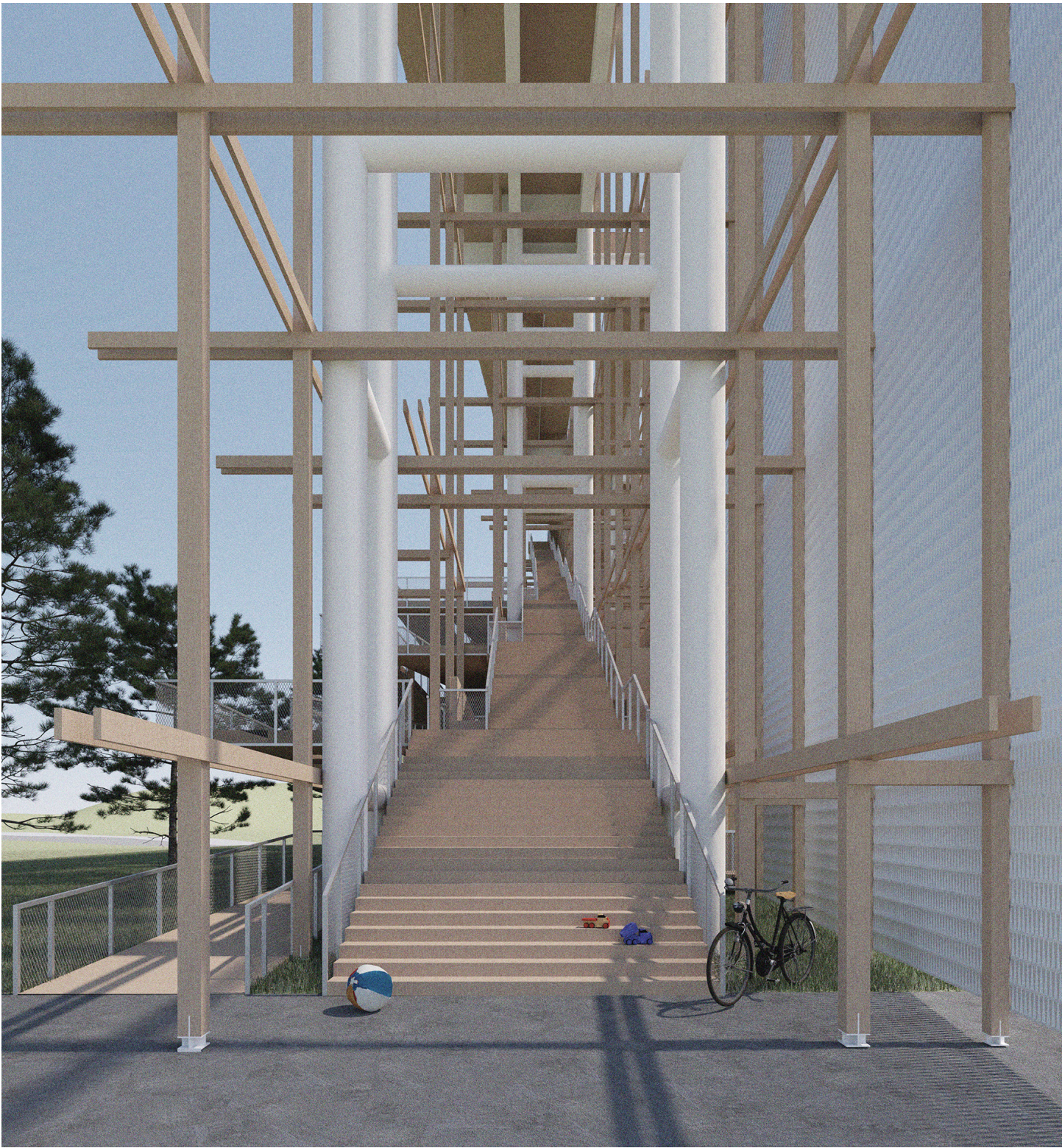
Left: A continuous run of stairs connects from the ground level up to the 90' tall platform. The stair is wider at the bottom and narrows at the top, providing space for gathering and events. Each landing of the stair connects with the ADA accessible ramp that leads to the housing and connects to the platform at the top.
