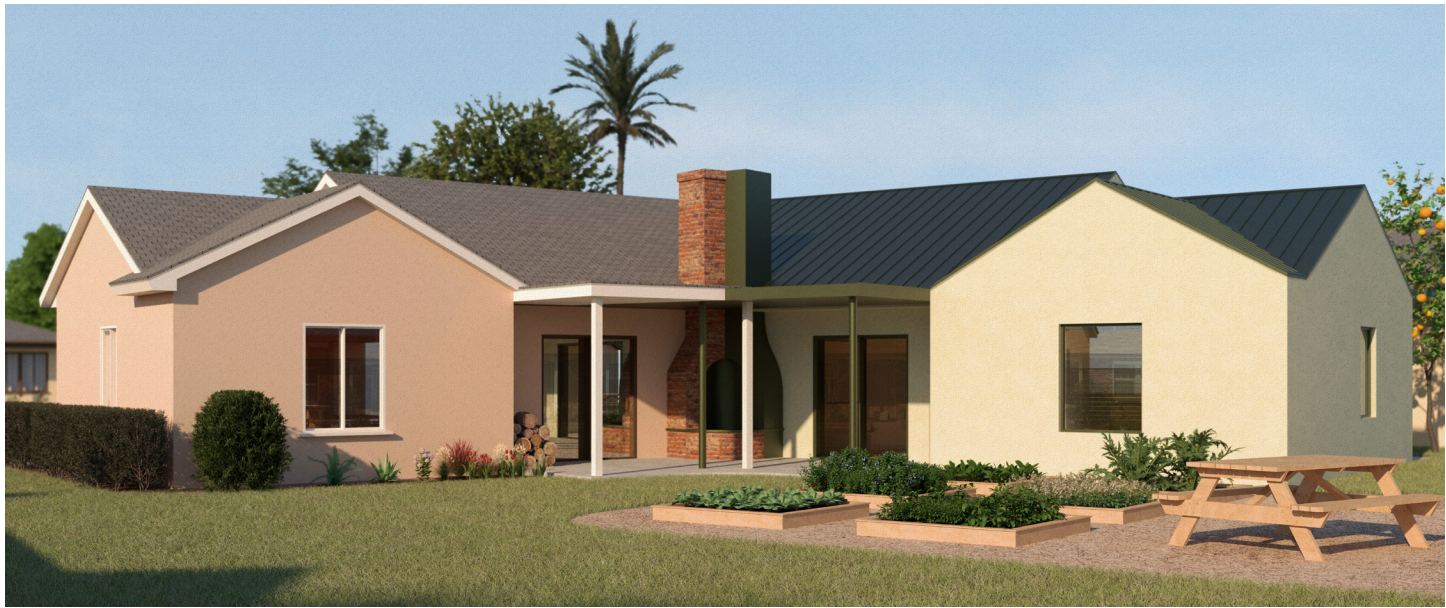
Above: One of the first strategies for Duplexing an existing single family house is called the Self Duplex. Working within the setbacks of the lot, the existing house is mirrored at an angle which results in an overlap of interior spaces that can be resolved into flexible and shared spaces.
