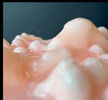
70% Ecoflex & 30% Brushable Brush Method: Normal Layer Number: 4 Color: Original color after mixing Transparency: Medium Flexibility: High
