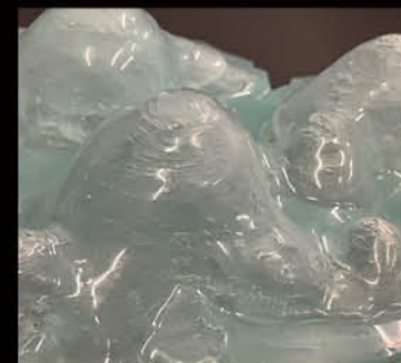
80% Ecoflex & 20% Brushable Brush Method: Normal Layer Number: 2 Color: Green pigment Transparency: High Flexibility: Too High
