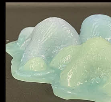
70% Ecoflex & 30% Brushable Brush Method: Mold Upside Down Layer Number: 4 Color: Green, blue, and purple pigment Transparency: Low Flexibility: Medium
