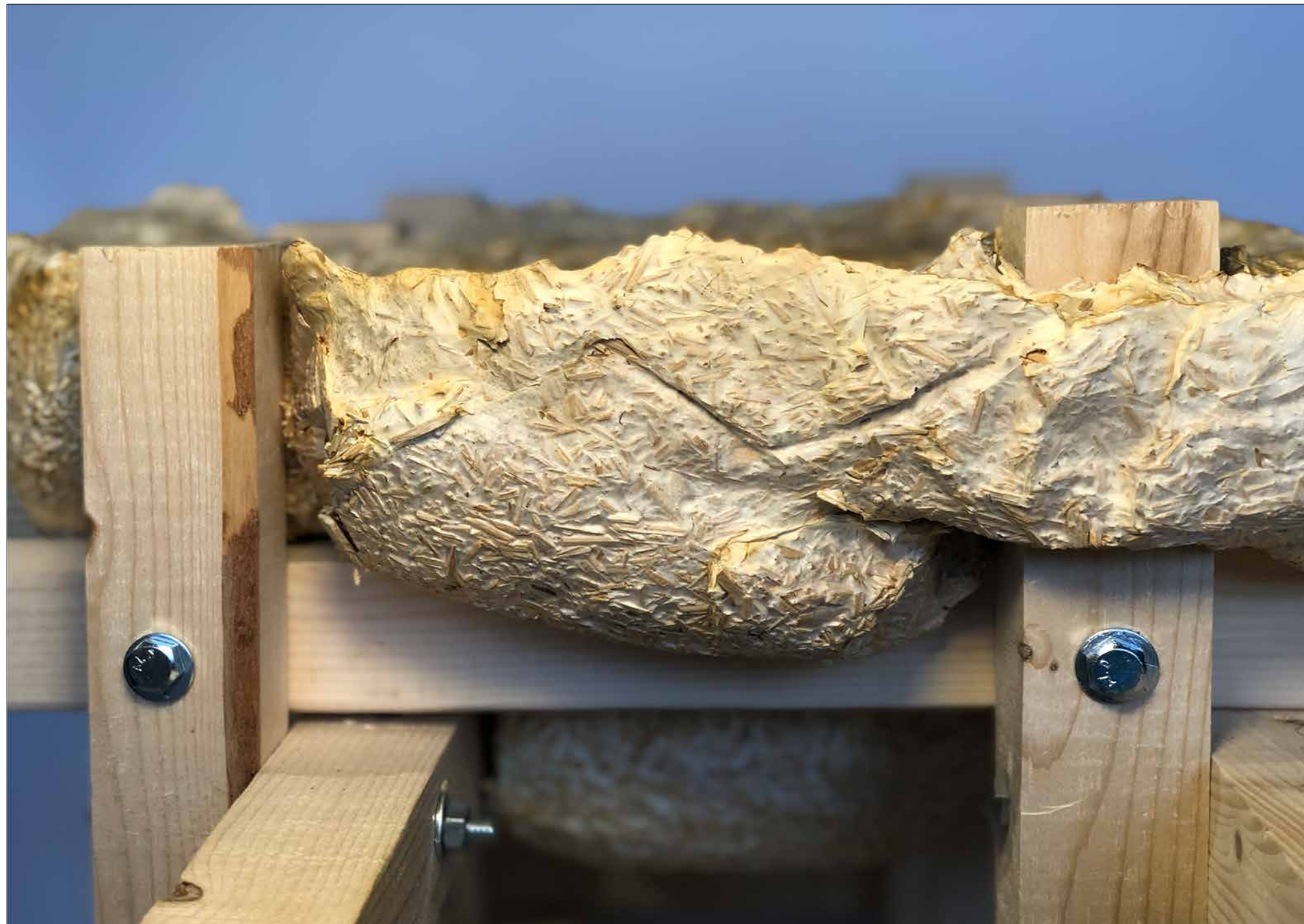
1' = 1' Study Model - Reishi Mycelium, Wood, Metal Bolts
