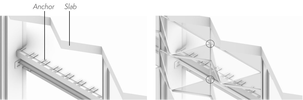
Anchors connecting slab to vertical member of curtain wall
