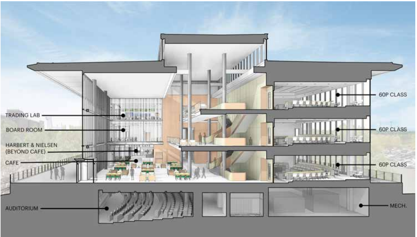
Perspective Section of Collat School Building Section through Atrium, Grand Stair, and Classrooms Looking West
