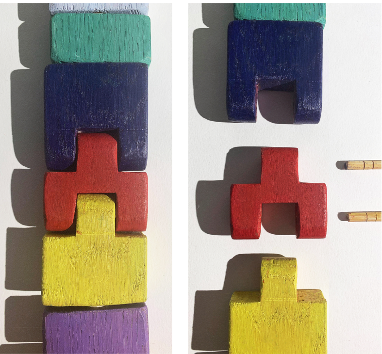
These joints resemble a finger joint in wood working. They are held together, pressure fit by a dowel. The pieces are rounded in order for them to rotate around each other freely.
