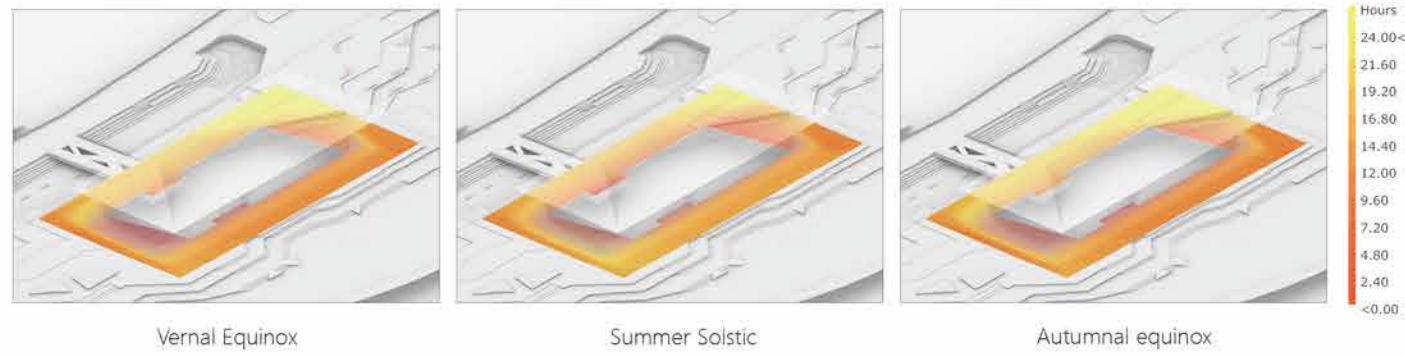
Self-shading effect of the floating roof
