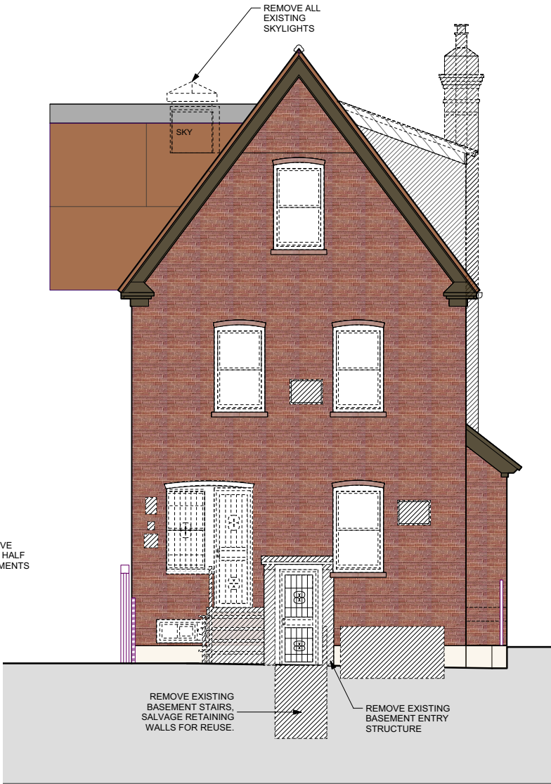
3 DEMO ELEVATION - REAR - WEST Scale: 1/4" = 1'-0"
