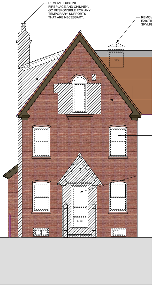
1 DEMO ELEVATION - FRONT - EAST Scale: 1/4" = 1'-0"
