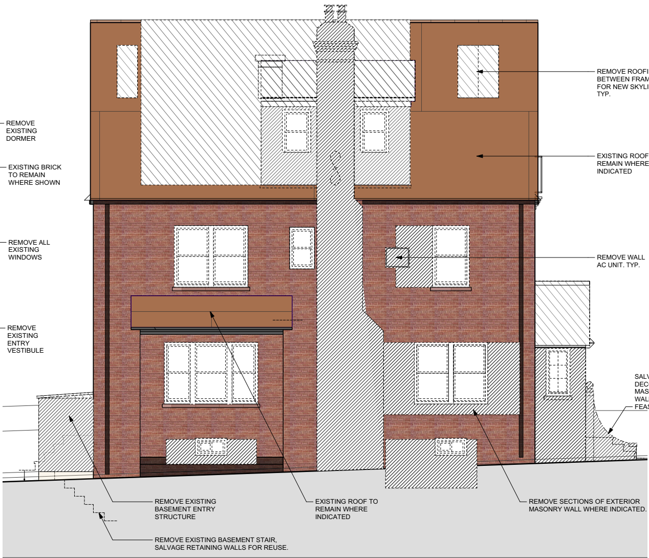
2 DEMO ELEVATION - SIDE - SOUTH Scale: 1/4" = 1'-0"
