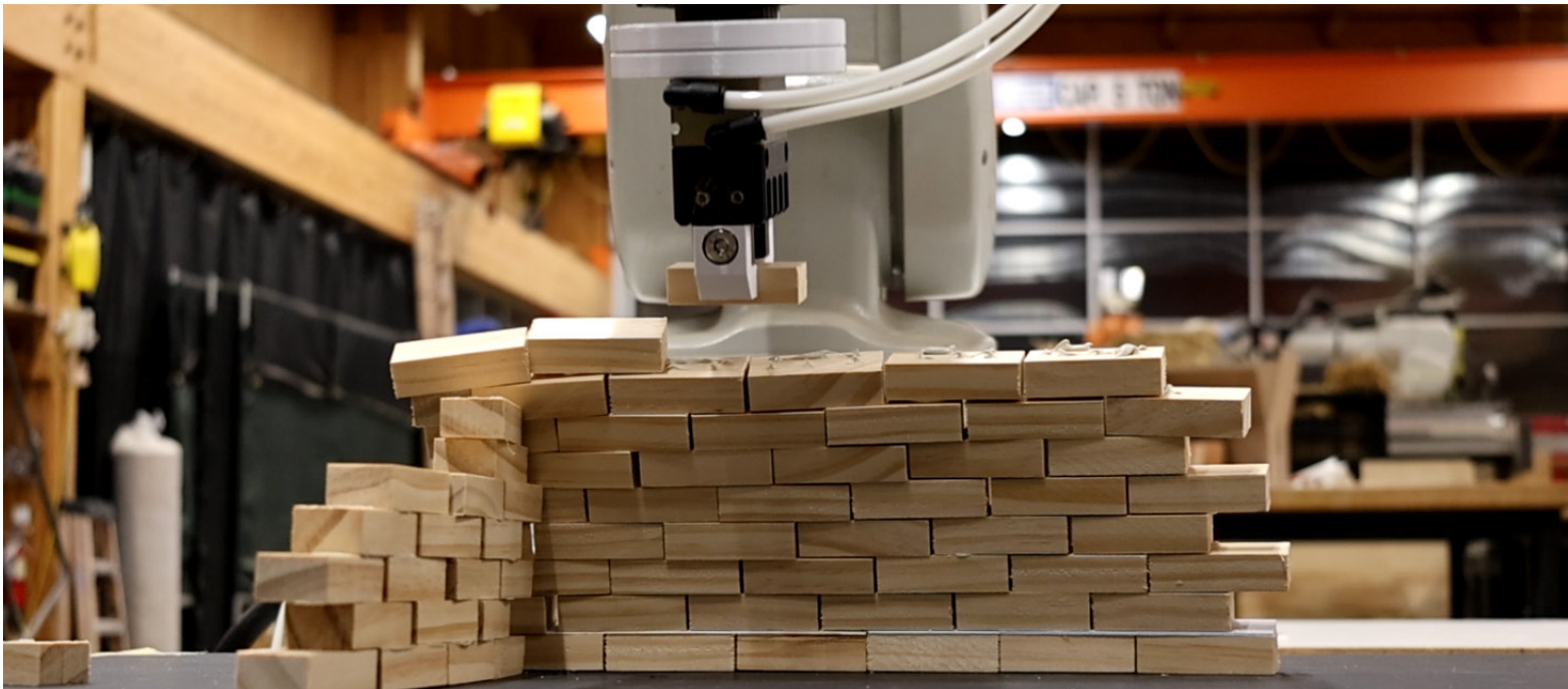
Machine Assembled Prototype for the Double-Curved Wall
