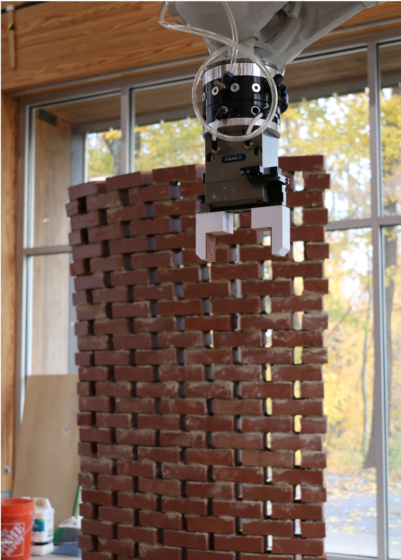
Robotic Arm used for Full-Scale Fabrication of the Double-Curved Wall
