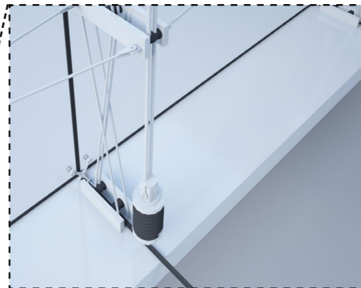
Cable structure of glass facade and damper
