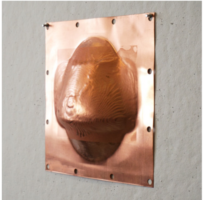
12 form E copper sheet 0.021" spiral machining with step-down silk-print texture
