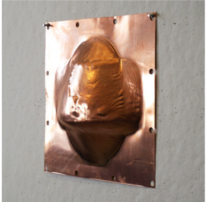
11 form E copper sheet 0.021" spiral machining with step-down
