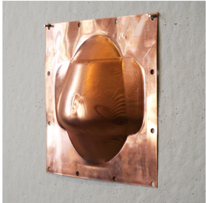
09 form D copper sheet 0.021" spiral machining with step-down
