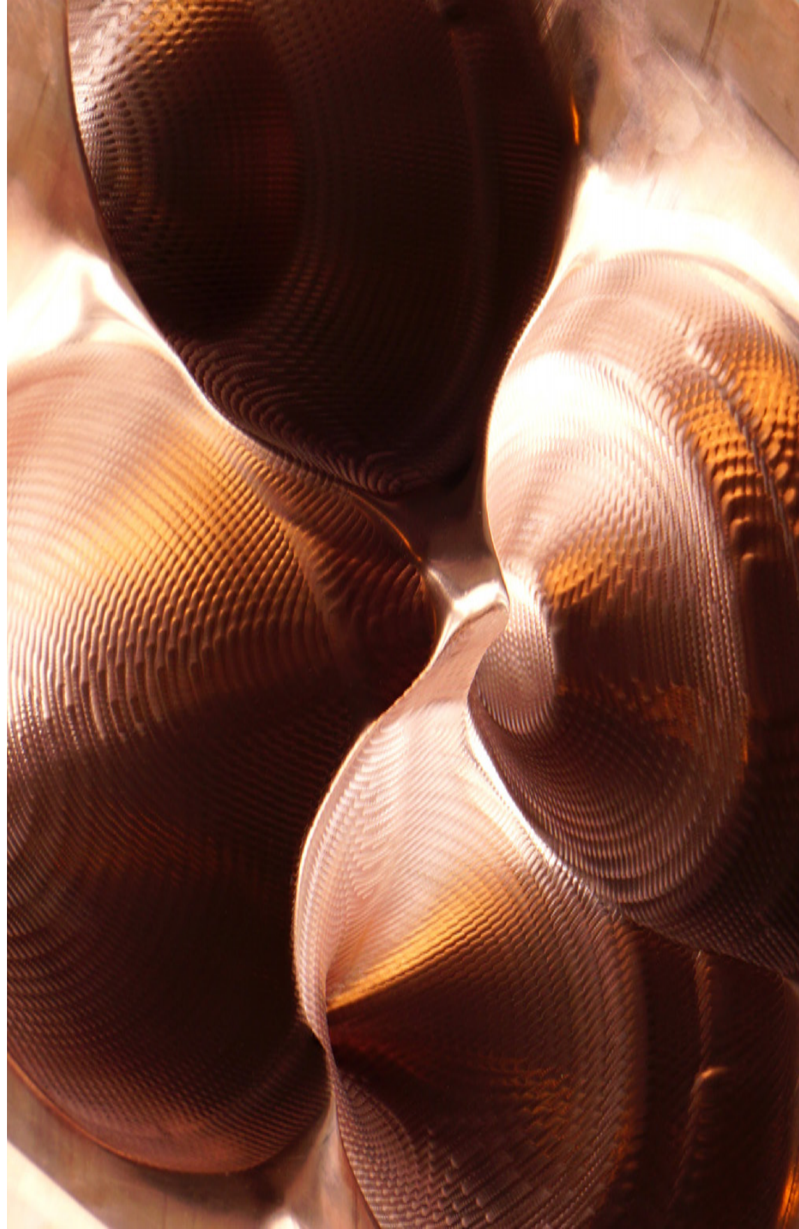
A quarter of the Utah Teapot "rendered" by single point incremental forming.
