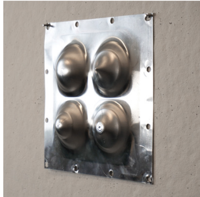
03 form B aluminum sheet 0.032" horizontal machining without step-down
