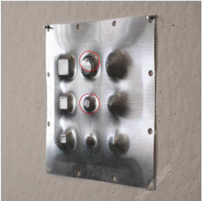
13 form A (zx0.75) aluminum mesh 0.032" 0.0625" Hole 30% open area horizontal machining without step-down error: thin material → material tore up
