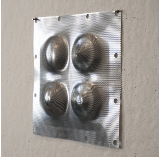
14 form B (zx0.75) aluminum mesh 0.032" 0.0625" hole 30% open area horizontal machining without step-down
