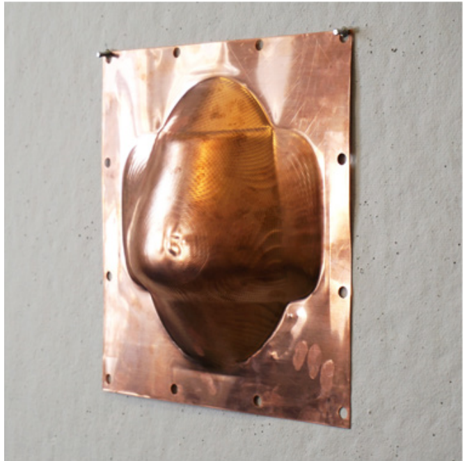
10 form D copper sheet 0.021" spiral machining with step-down off-center
