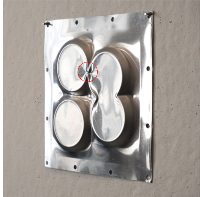
05 form C aluminum sheet 0.032" horizontal machining without step-down error: pinching effect → tooling ball broke
