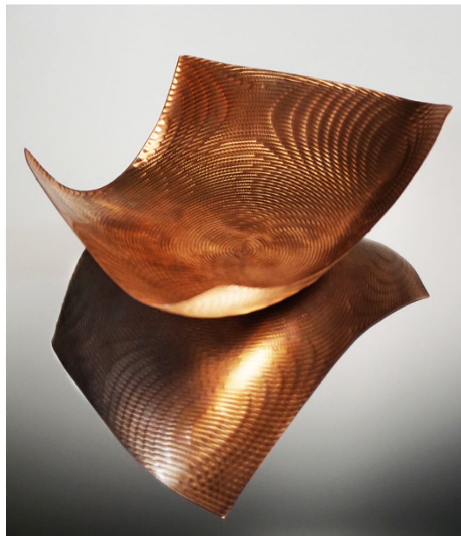
A quarter of the Utah Teapot "rendered" by single point incremental forming.
