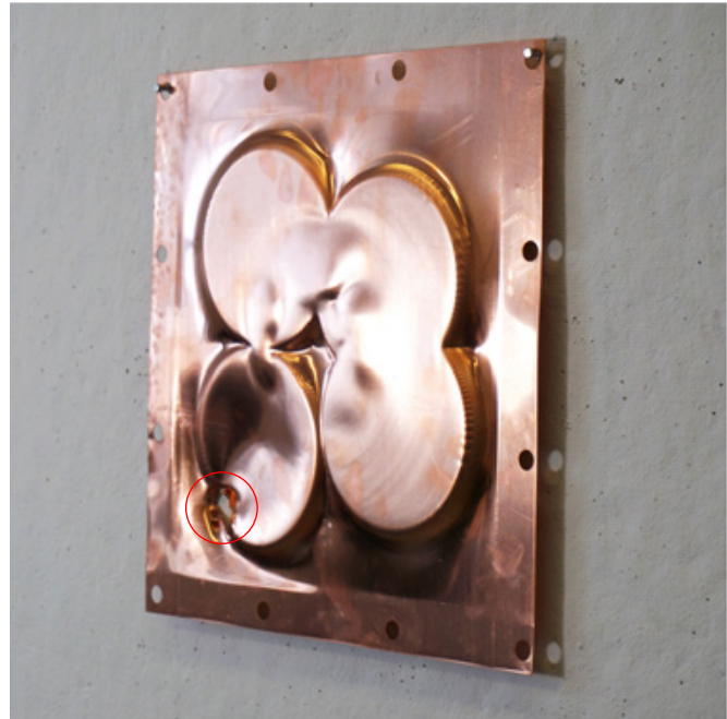
06 form C copper sheet 0.021" spiral machining with step-down error: no touch off → material tore up
