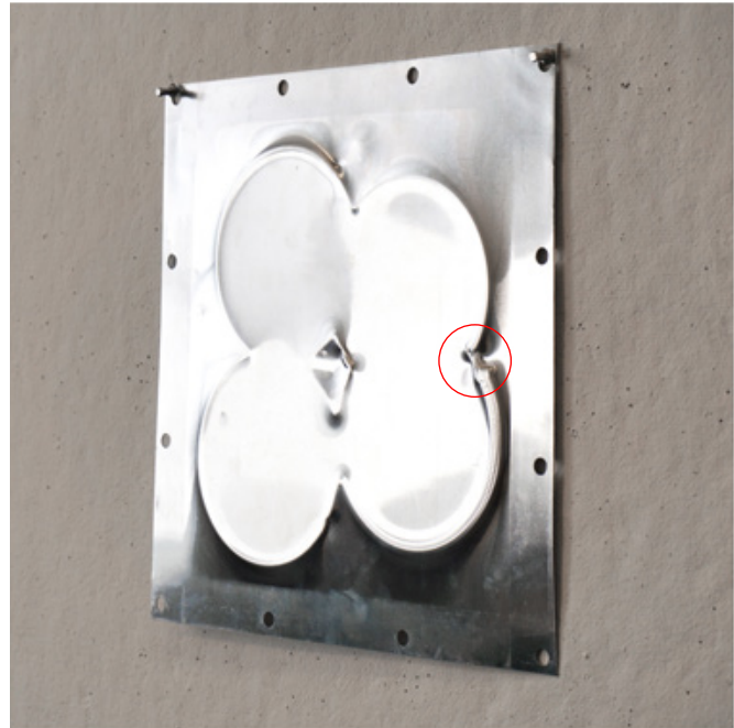
04 form C aluminum sheet 0.032" horizontal machining without step-down error: mold misplaced → tooling ball broke
