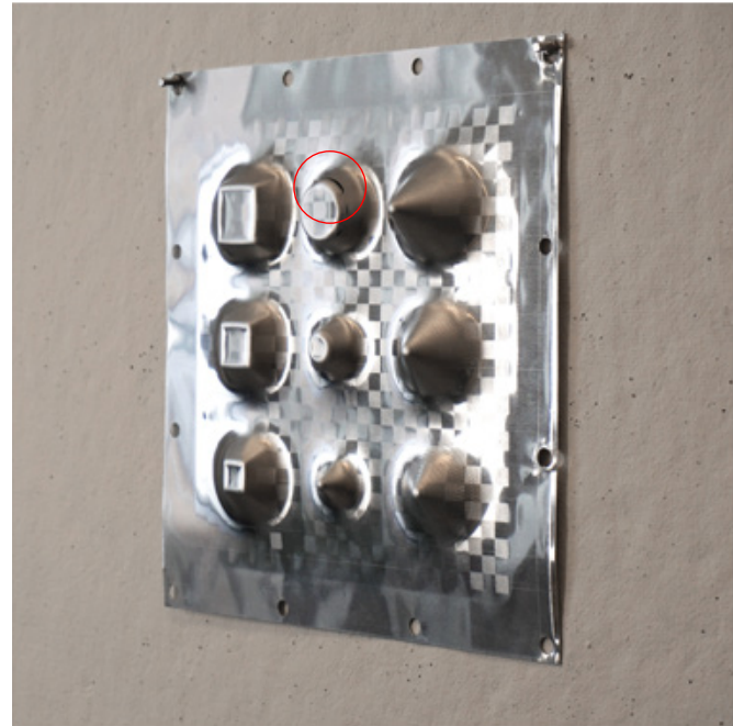
01 form A aluminum sheet 0.032" horizontal machining without step-down error: thin material → material tore up
