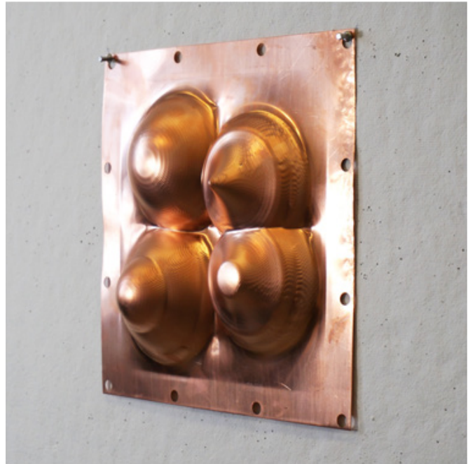
07 form C copper sheet 0.021" spiral machining with step-down
