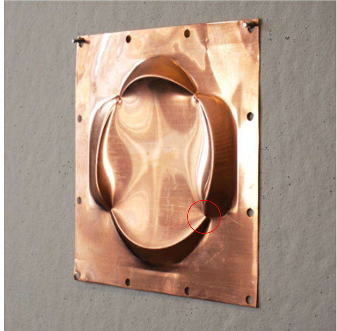
08 form D copper sheet 0.021" spiral machining without step-down error: pinching effect → tooling ball broke
