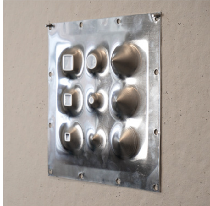
02 form A aluminum sheet 0.032" horizontal machining without step-down
