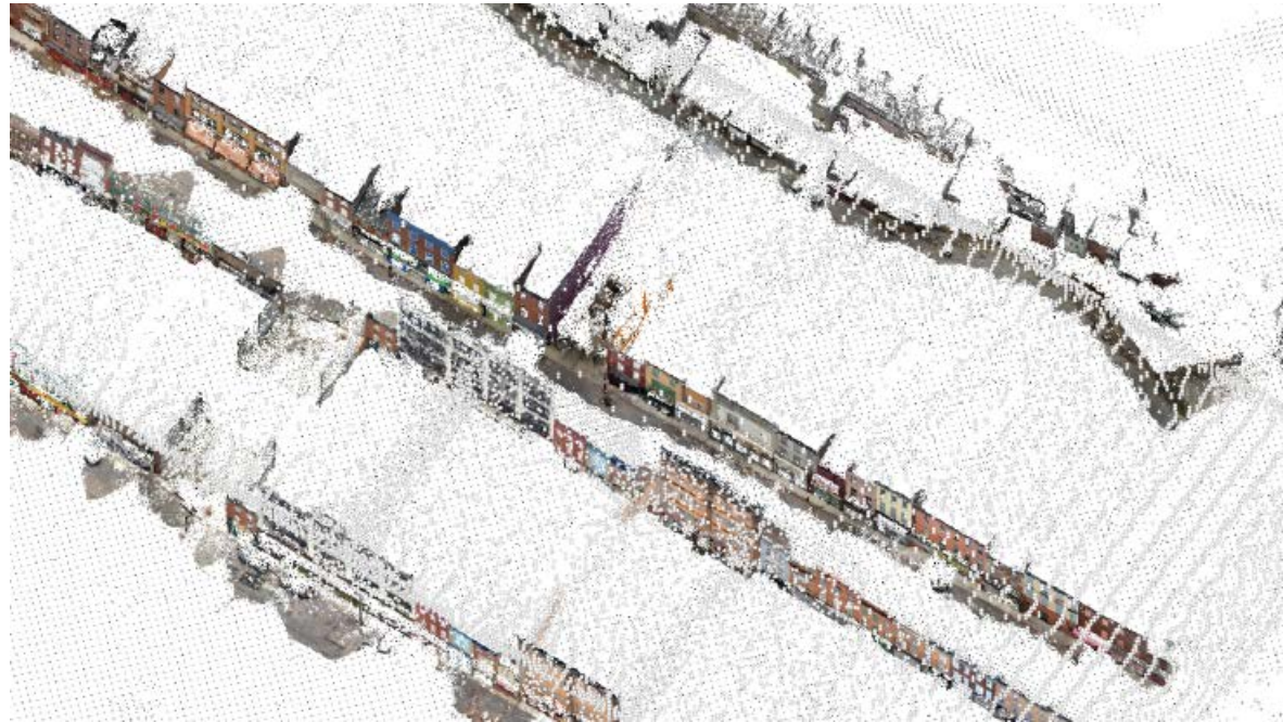
Photogrammetry of the Existing Facades
