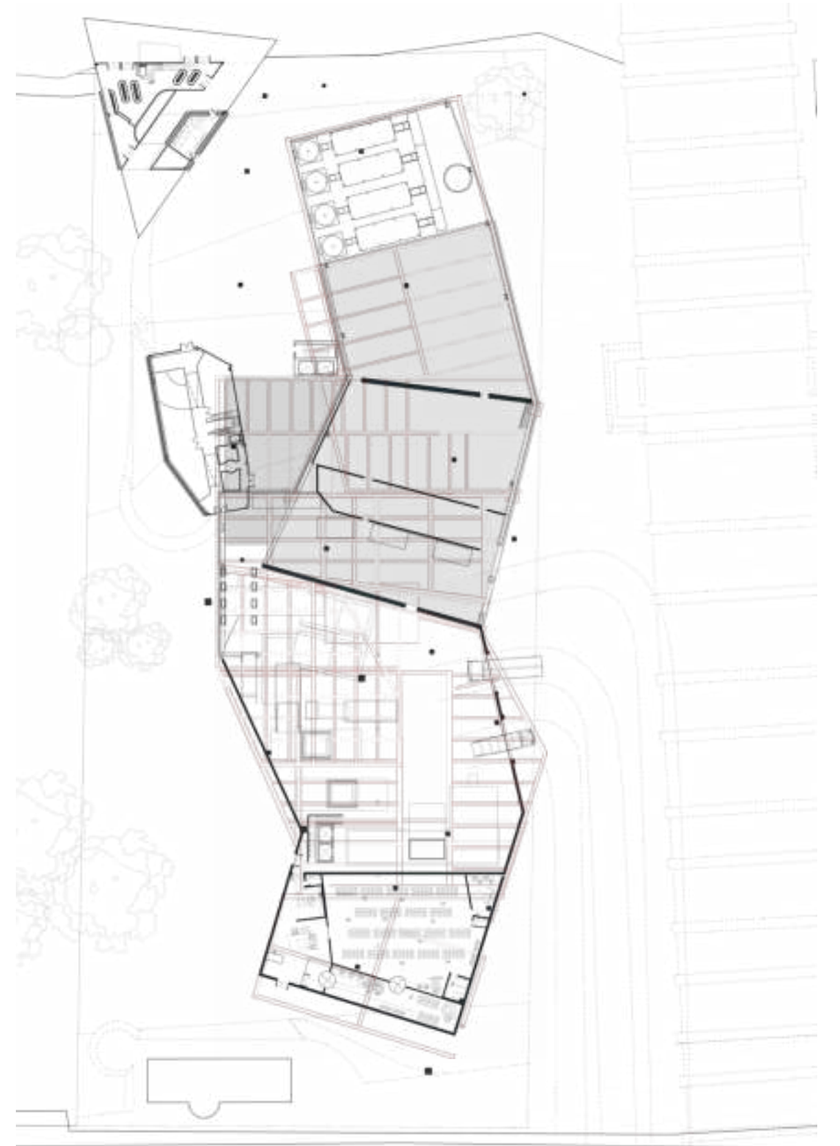
Ground Floor + Structural Framing
