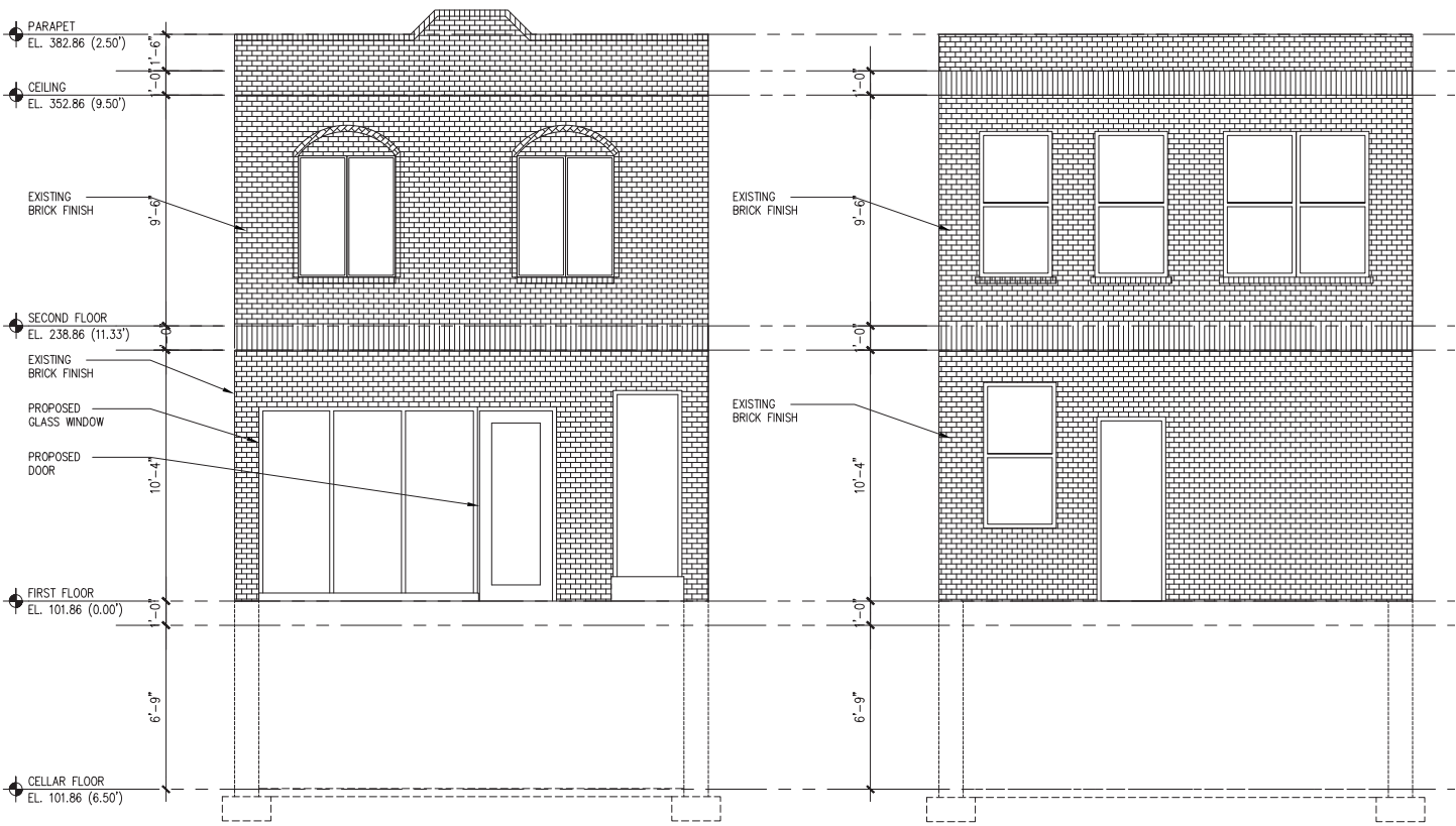
FRONT SIDE ELEVATION SCALE: 1/4" = 1'-0"
