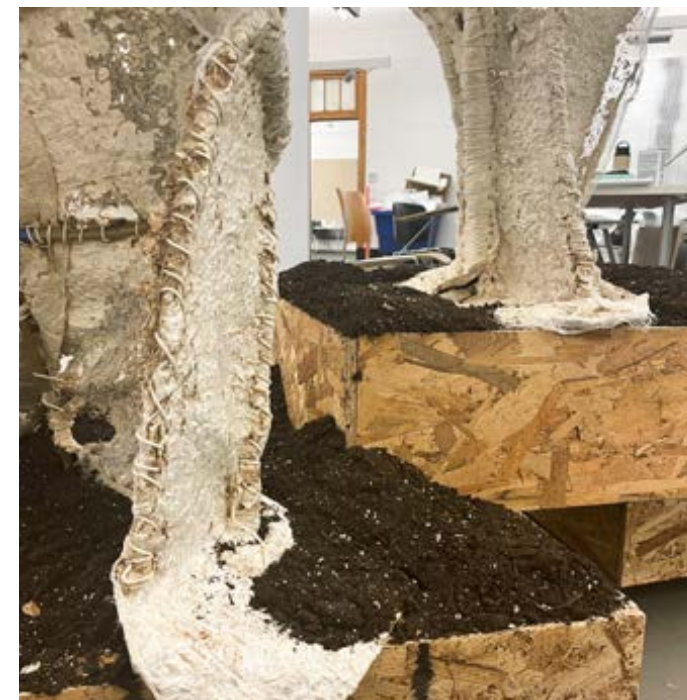
GROWING MYCO-FABRIC ON BAMBOO STRUCTURE
