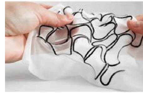
0% - 100% Ratio behavior : multi-directional stretch
