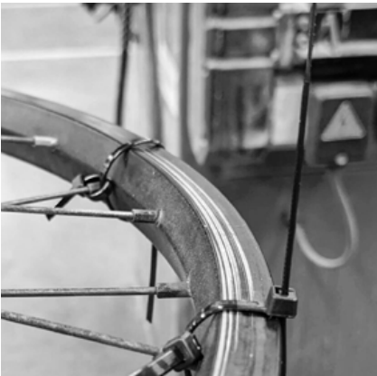
Closeup of the zip tie solution. The sound produced did not compliment the feel we had in mind for the bikestriment.
