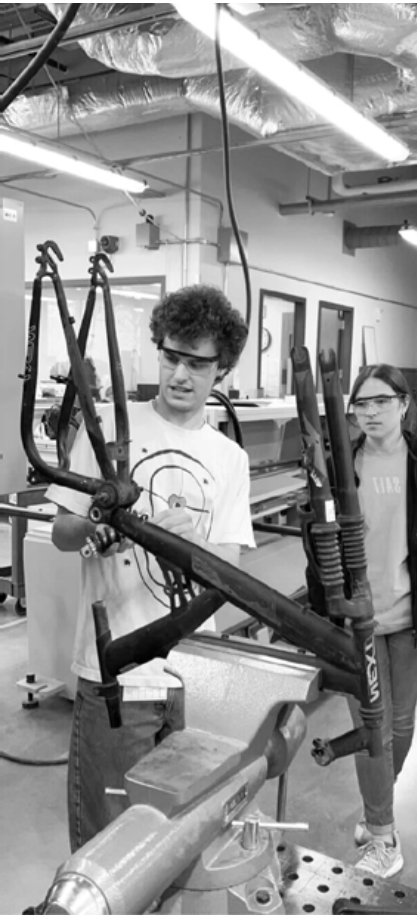
Reserving our budget for later stages of the project, we first secured an abonded bike from a dumpster to strip down and understand. This prototype used the bikes existing suspension joint to change the tension and pitch of the strings.
