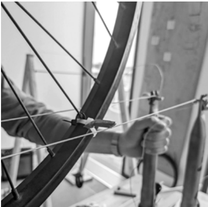
Initial prototype struck the strings with zip ties and guitar picks fastened to the rims of the bike wheel.
