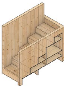
Embed Storage (Under Stair) Toilet
