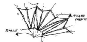
Folded plates are used for roofing type according to design and radial concept.
