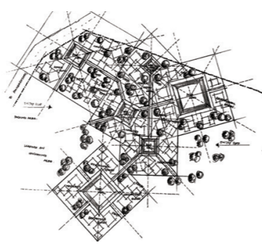
Defining the axis of the waterbodies through pathways creates visual continuity, movement, spatial orientation, and unifies site design.
