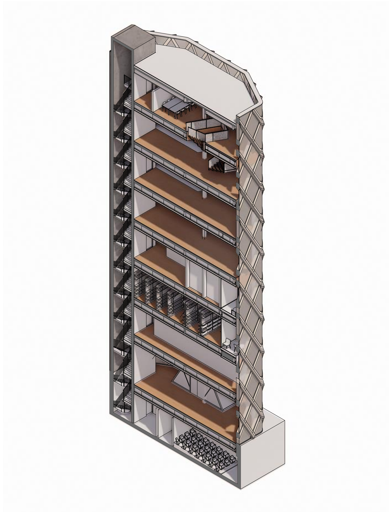
Building Assembly Section
