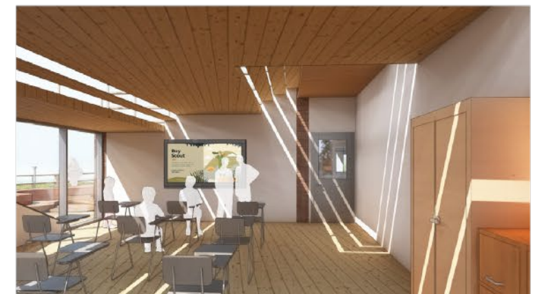
Classroom - the stepped roof with skylights between the risers creates a dynamic lighting scheme
