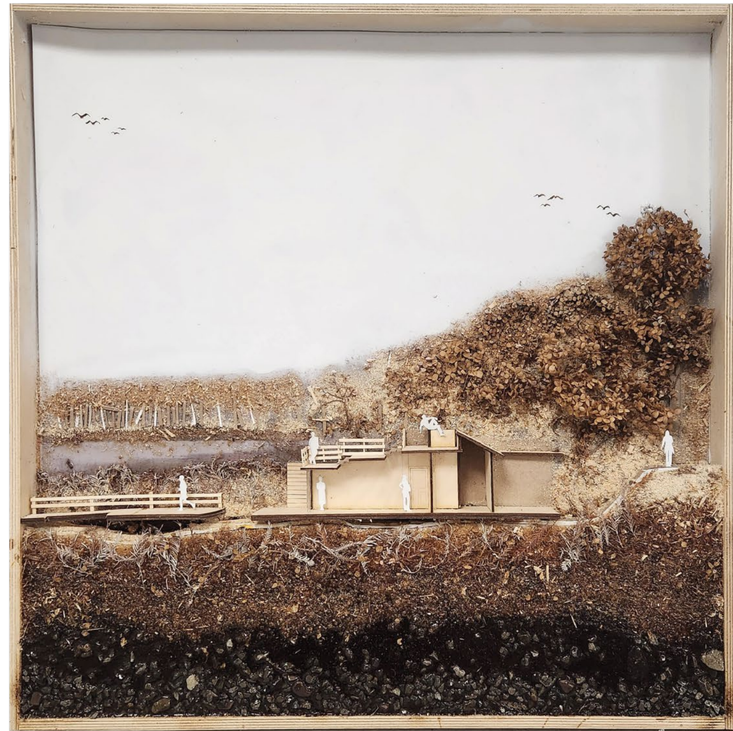
A forced perspective physical model showing a section of the nature center. The different levels step down one by one, taking the visitor from the campgrounds down to the boardwalk level while using the roof as a panoramic viewing platform.
