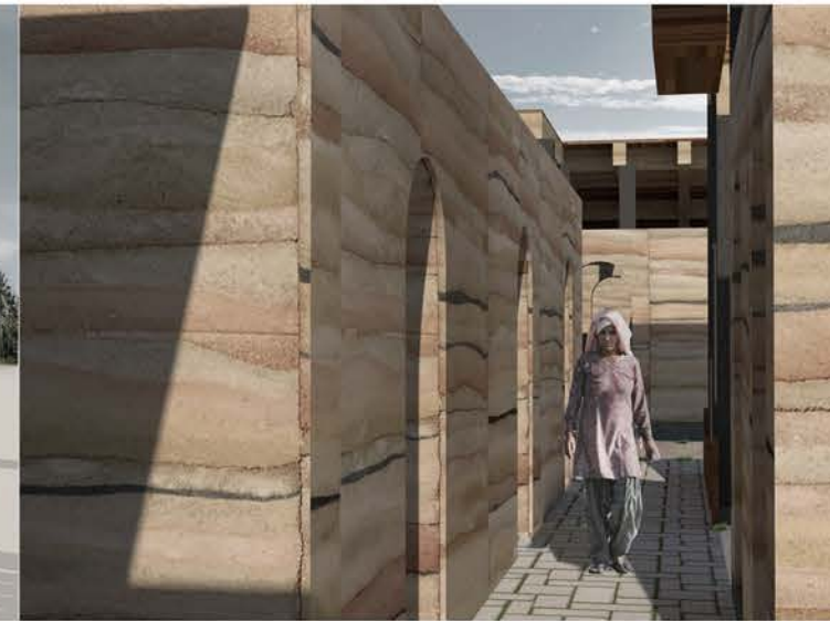
View depicting internal lanes with structures placed rather close to one another to ensure maximum sciography and create a better microclimate.
