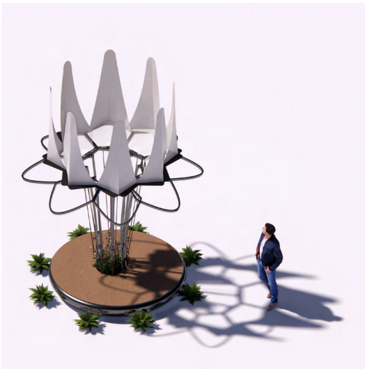
When the user is not using the canopy, it is used for rainwater collection
