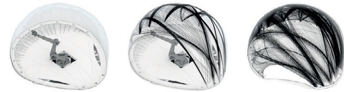
Conceptual Fabrication Strategy: 1. Inflated pneumatic membrane 2. Robotically reinforce membrane with carbon fiber from inside 3. Stable composite shell © ICD/ITKE University of Stuttgart.
