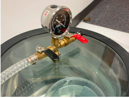
6. De-gas resin at 25psi in multiple increments
