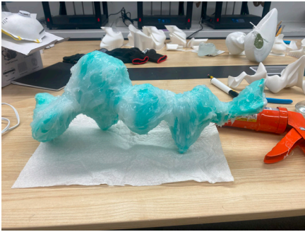
4. Add layer of silicone sealant, preventing leaks
