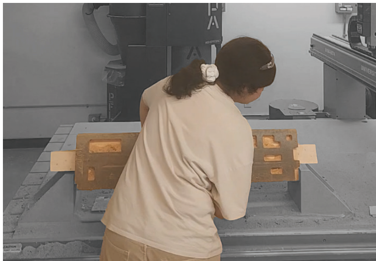
▲ Flipping the stock after a face finishes milling
