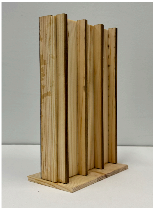
Model of structural concept: Pre-fabricated rock wall casts, with integrated wall joists for interior walls. Large aggregates are poured into the cast, along with stratified layers of strong mortar, creating the structural outer walls. The outside-facing mold is then removed, leaving behind a thick, self-insulating stone wall, and interior wall joists, ready for drywall. The system aims to cut down on the need for insulation means and labor.
