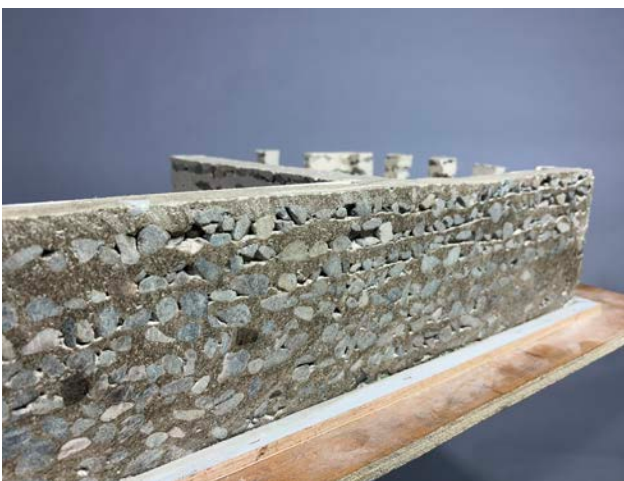
Townhouse sectional model: Pre-fabricated rock wall casts, with integrated wall joists for interior walls. Large aggregates are poured into the cast, along with stratified layers of strong mortar, creating the structural outer walls. The outside-facing mold is then removed, leaving behind a thick, self-insulating stone wall, and interior wall joists, ready for drywall. The system aims to cut down on the need for insulation means and labor.
