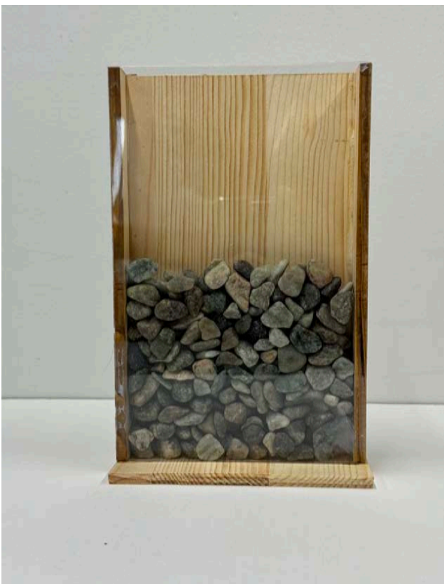
Model of structural concept: Pre-fabricated rock wall casts, with integrated wall joists for interior walls. Large aggregates are poured into the cast, along with stratified layers of strong mortar, creating the structural outer walls. The outside-facing mold is then removed, leaving behind a thick, self-insulating stone wall, and interior wall joists, ready for drywall. The system aims to cut down on the need for insulation means and labor.
