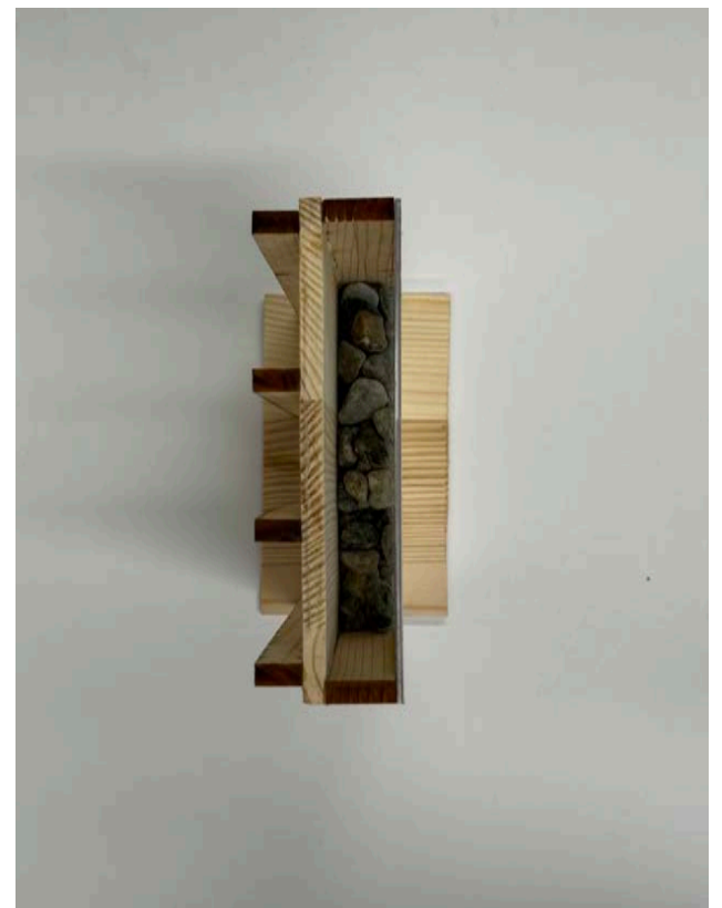
Model of structural concept: Pre-fabricated rock wall casts, with integrated wall joists for interior walls. Large aggregates are poured into the cast, along with stratified layers of strong mortar, creating the structural outer walls. The outside-facing mold is then removed, leaving behind a thick, self-insulating stone wall, and interior wall joists, ready for drywall. The system aims to cut down on the need for insulation means and labor.
