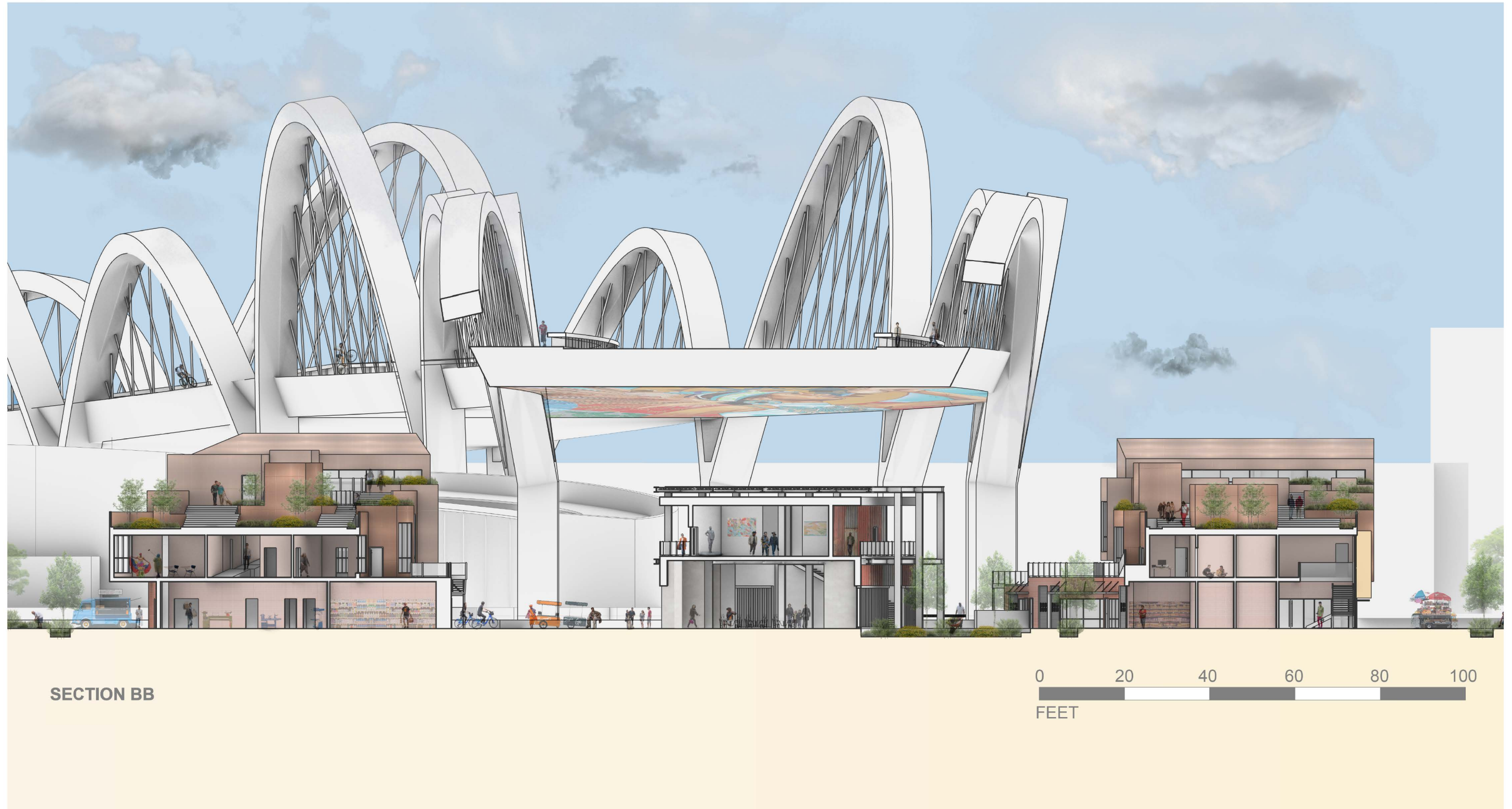
The section reveals the vertical organization of public, maker, and educational spaces beneath the 6th Street Viaduct, framing protected plazas while maintaining visual and physical connections to the bridge and river corridor.
